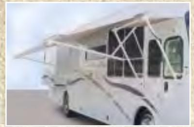
*Electric main awning with wind sensor slide-out covers and window awnings.*
