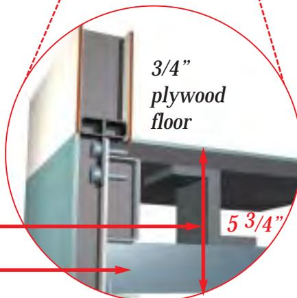
3" steel framed vacuum bonded basement floor
